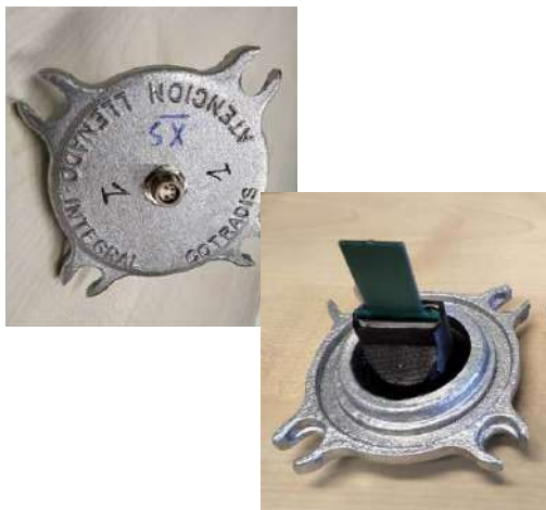
Monitoring of oil dielectric constant in Transformers
